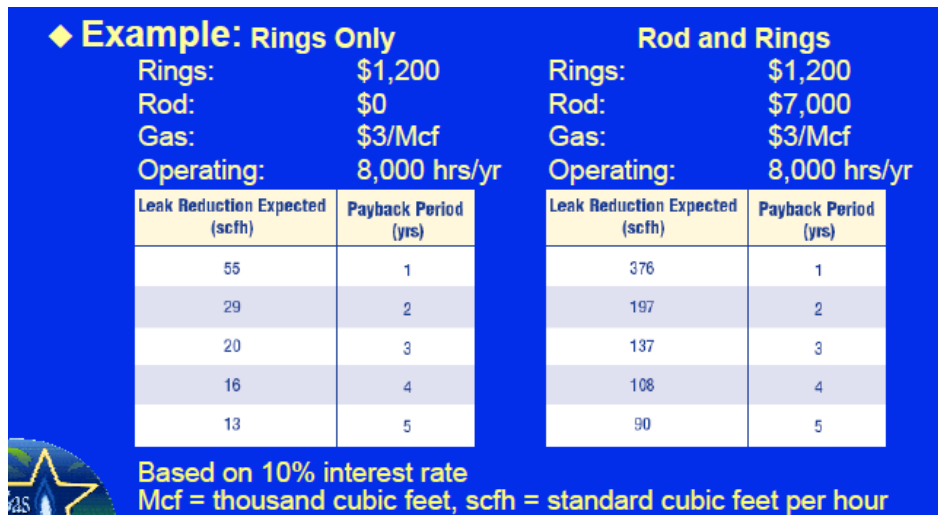
Figure 60. Example of replace packing and rods when cost-effective
